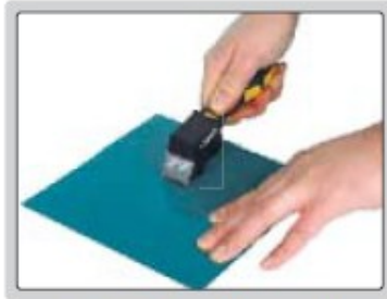
step 1: make grid cutting on surface
